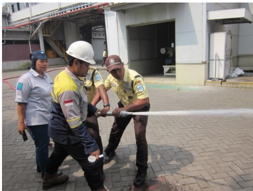
Percobaan operasional hydrant percobaan tes pressure pompa hydrant
