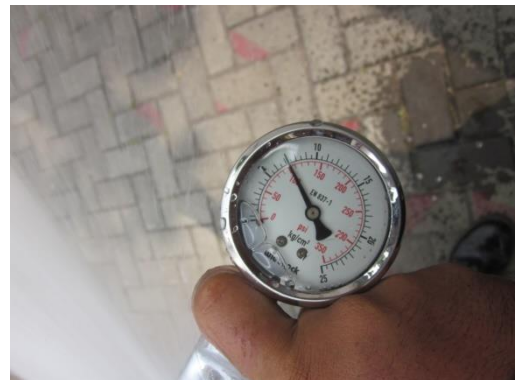
Percobaan operasional hydrant percobaan tes pressure pompa hydrant
